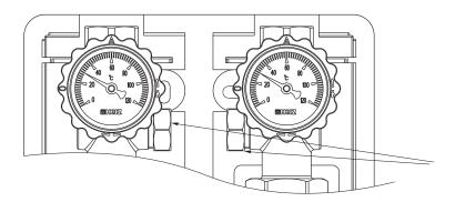
Overflow valve can be installed on DN20/25/32 HERZ PUMPFIX pump group.
