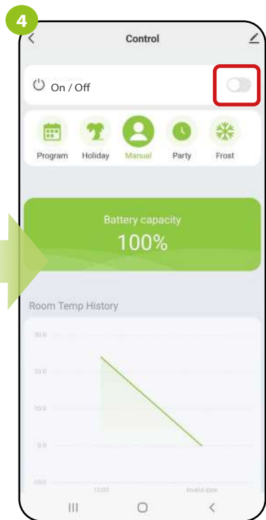
When the „Power” slider is grayed out, then the thermostat is off...
