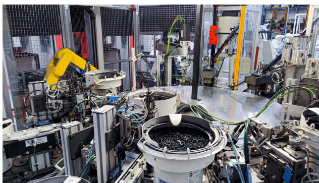
Figure 27 Assembly station rotating table.
