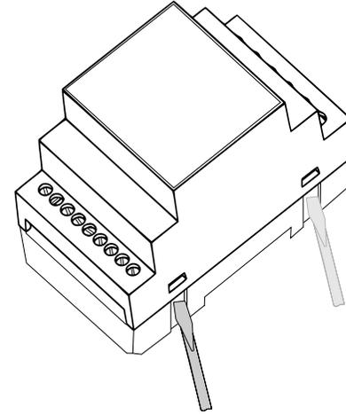
To open the casing of the module, you need to pry all the hooks (with a flat screwdriver) and then carefully remove its upper part.
