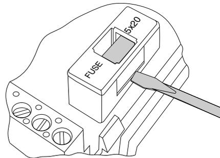
Using a flat screwdriver, pry the fuse holder, replace the fuse, put the holder back in place and then snap the upper housing of the module.
