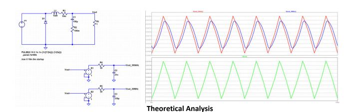
The component of the output ripple is built by the output current and the equivalent series resistor of the output
