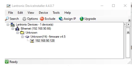
You can also find the IP by typing "arp -a" in the command prompt in windows. Check the MAC address of the device (label on the device or in calibration protocol). The IP on the left side of the MAC address is the current IP of the device.
