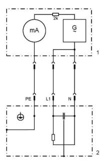
Note: The illustration shows the measurement method for two-phase power supplies. In the three-phase version, phase N is replaced by L2 and/or L3.
