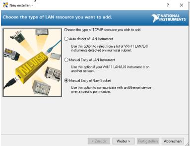
Now the IP address and the port number (10001) are entered. The connection can be checked with Validate.
