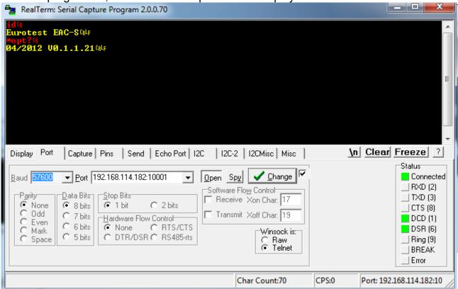
Now enter the IP address in the form xxx.xxx.xxx.xxx:10001 in the "Port" tab and press the Open button. Commands can now be sent to the unit in the terminal field.
