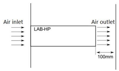
Air inlet volume = 310m³/h per 7.5kW module (maximum value)
