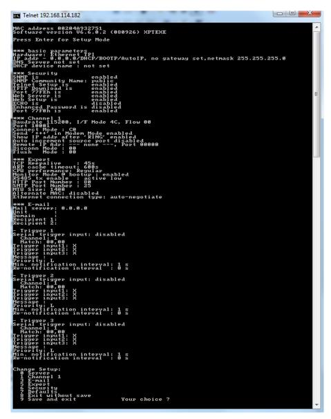
To set the IP address permanently, we need the menu "Server" (selection 0). Now the IP address is entered again (finish all four groups of digits with the enter key). The other settings remain unchanged (simply press the enter key). Then the configuration is saved and ended by selecting menu item 9.
