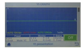
In this representation, the current I, the voltage U and the power P are plotted on the Y-axis and the time t on the X-axis. The resolution is set automatically here. In operation, the graph is updated every 0.5s and thus runs from right to left. In standby, the recording is stopped.
