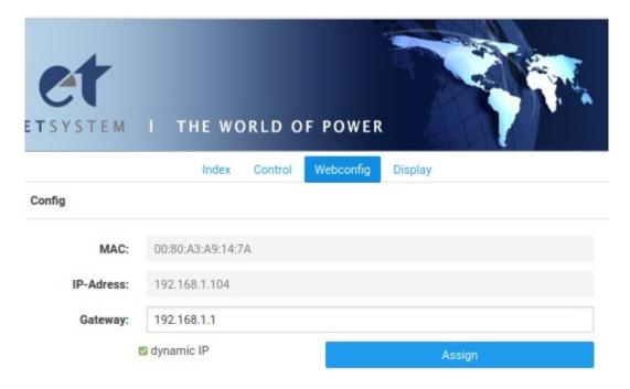
To configure the IP, uncheck Dynamic IP and enter the IP address. After confirmation via Assign, the new (static) address is saved. It is possible that the connection will be interrupted shortly because the interface is performing a reset.
