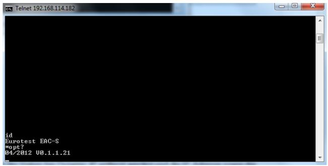
When controlling the units via port 10001, the user interface must not be started in a browser! As an alternative to Telnet, many terminal programmes have the option of establishing a TCP/IP or Telnet connection.
