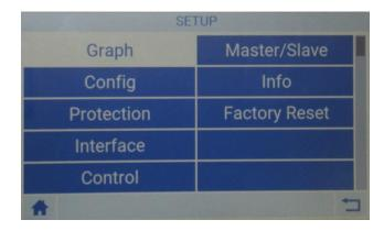
By pressing the "Mode" button or the upper rotary encoder in standby, the item "Config." appears at the top of the screen. Clicking on this point or pressing the upper rotary encoder again takes you to the settings.
