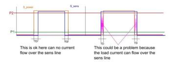
The circuit breaker (S\_power) must be closed when starting before the Sens (S\_sens). When switching off, the Sens must first be opened and then the circuit breaker can be opened. Otherwise, a current flow may occur across the sensing line, and this may be particularly critical when disconnecting.
