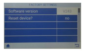
Here the unit can be reset to factory settings. This includes all changes made to the unit by the customer (note: the controller values are also deleted).
