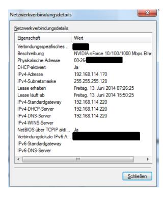
In this example, the IP address of the computer is 192.168.114.170 The IP address of the server is 192.168.114.220 The subnet mask is 255.255.255.128
