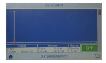
In this representation, the current I is plotted on the Y-axis and the voltage U on the X-axis. The red frame represents the maximum limits determined by the set values. A red X symbol represents the current operating point.
