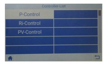
Here, the digital PID controllers of the individual modes can be readjusted and thus adapted to the respective application. The values to be set range from 0 to 9.9999. The higher the value set, the greater the range of influence of the respective controller.
