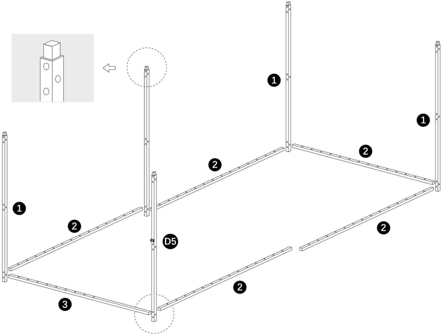
Note: No.3 is pipe with half pre-drilled holes
