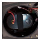
④ Secure the battery with Velcro straps and plug in the power cord.
