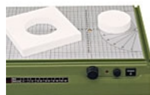
Crosscuts are achieved by means of a simple, yet efficient solution: secure to table with tape, it serves as a fixed centre.
