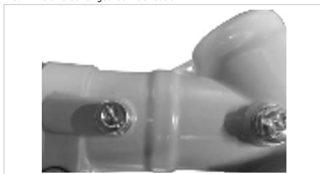
Pic. 21 Bolt holes for gearbox lubrication
