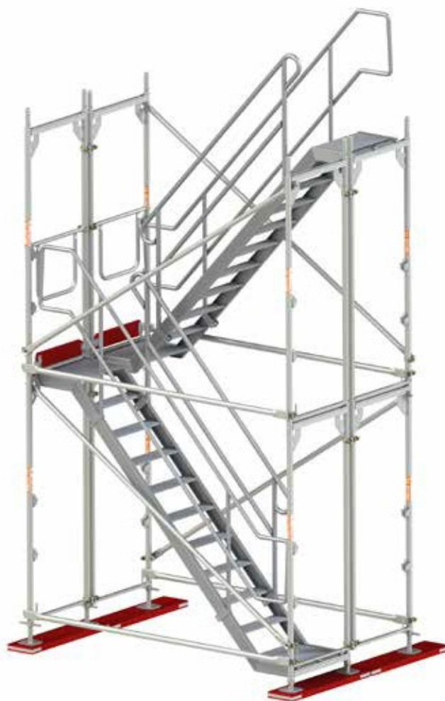
Fig. 43. Installation of the staircase, stage IV.
