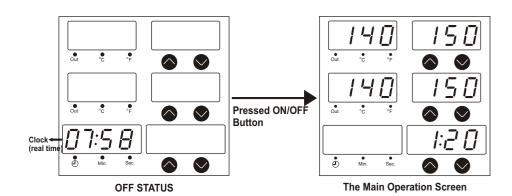
The cooked product is placed into  $\underline{th}$  oven. When the device is energized, it is opened in off status and [0758] clock appears. The on/off button is pressed to turns the main operation screen. The set values are values that existed before the device turns off. []. The temperature start button is pressed to start cooking. Set values can be changed while cooking. temperature stop button is pressed to stop cooking.
