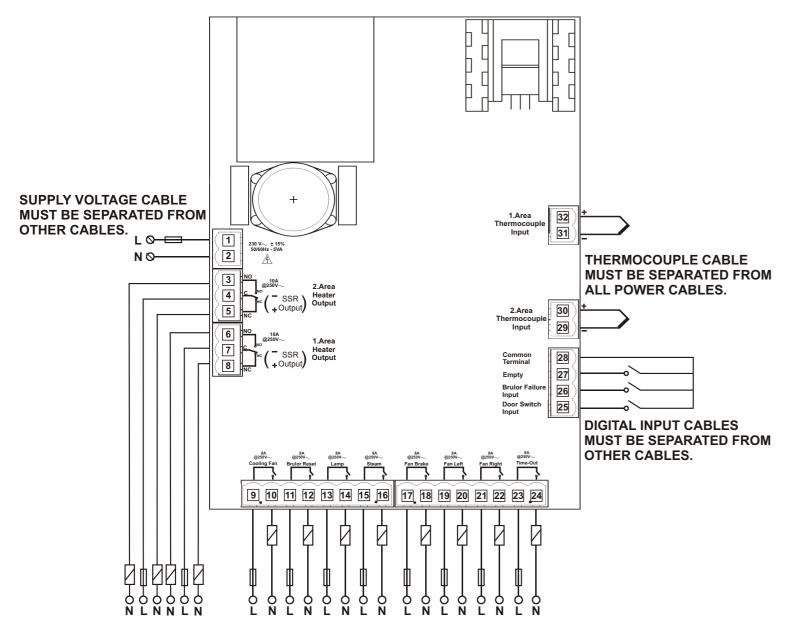
ALL POWER CABLES MUST BE SEPARATED FROM SENSOR, SUPPLY VOLTAGE AND DIGITAL CABLES.
