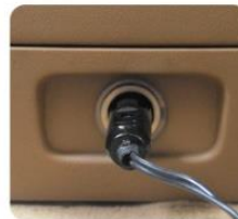
Insert 12V DC plug into cigarette lighter socket
