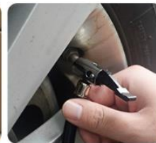
Connect to your tire, make sure air tightness
