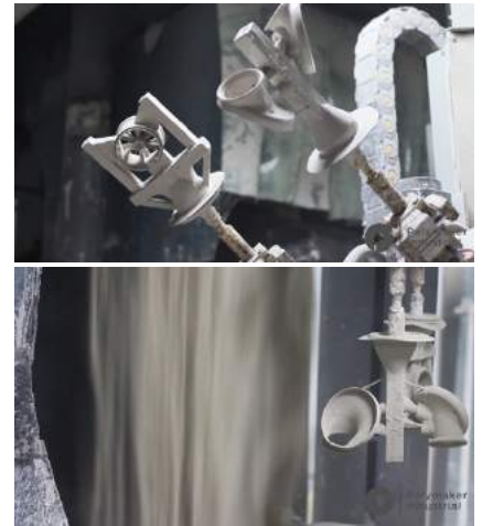
Figure 7. Make the ceramic shell
