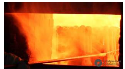
Figure 8. Sinter the ceramic shell and burnout
