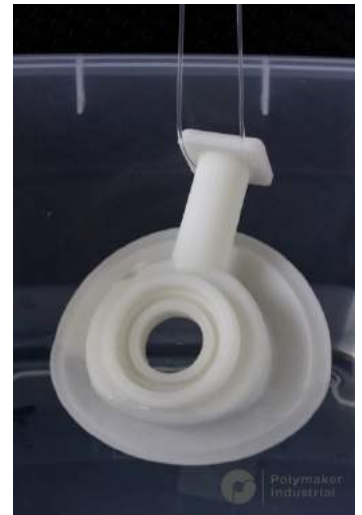
Figure 4. Dip the PolyCast™ pattern into isopropyl alcohol
