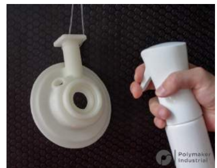
Figure 5. Spray isopropyl alcohol on the PolyCast™ pattern
