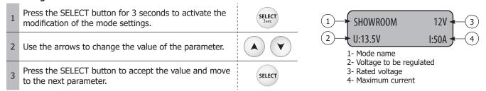
**Power limitation:** If the symbol «\*» appears next to the current setting (eg «I: 50A \*»), this indicates that the charger cannot deliver this current at the voltage set on the display. At this voltage level, the charger will be running at maximum power. However, this current could be delivered at lower voltage depending on the power output of the charger.
