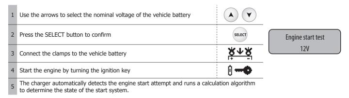
**Test result:** The charger indicates the minimum value of the battery voltage perceived during the engine start phase, as well as the status of the start system in the form of a gauge.
