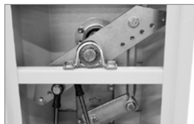
Metallic gear + shock resistant motor (ALT624K)
