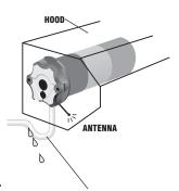
The motor cable should not act as a direct conduit for the water to enter the head of the motor (form drip loops).
