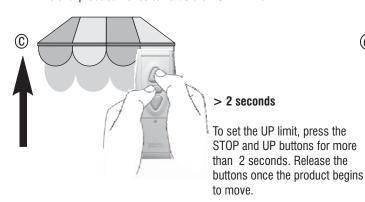
The awning goes up and reaches the completely closed position of the box.
