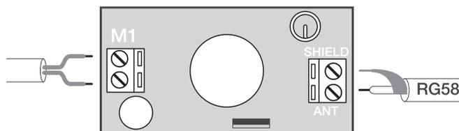
Connect the 24V flashing light output of the control unit to the terminal board M1 (see main connection layout).
