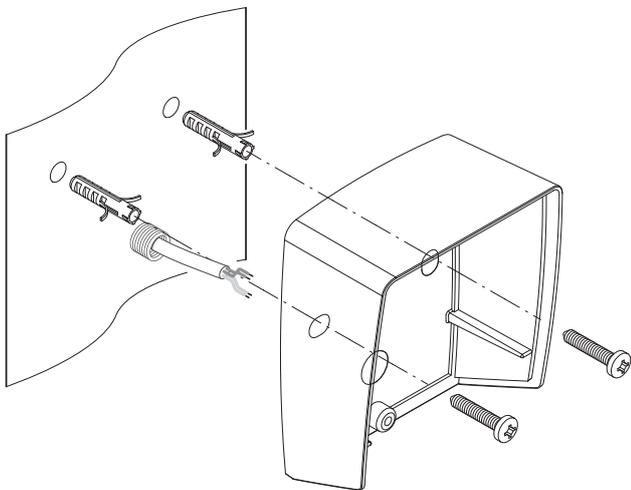
Using the support as a reference, mark and make two holes with diameter of 6 mm in a way that the lower hole corresponds to the set-up of the cables.
