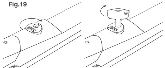
The gear motor is now released and the leaf can be opened and closed manually.
