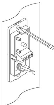
Make two holes with diameter of 6 mm in a way that the hole in proximity of the terminal board corresponds to the set-up of the cables. Insert the cable and fix the base of the photocell to the wall using the plugs and screws.
