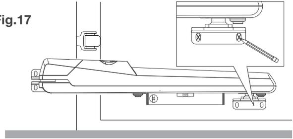
Also in this case the fixing devices will be selected on the basis of the material with which the leaf is made. Self-threading screws are used in the example in figure 18.
