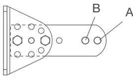
Select the position that corresponds to position "S" calculated in Table 1 of the "Choice of installation measurements" paragraph.
