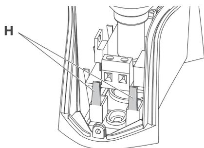
Remove the electronic circuit, pulling the two plastic tabs H outwards, thus releasing the board.
