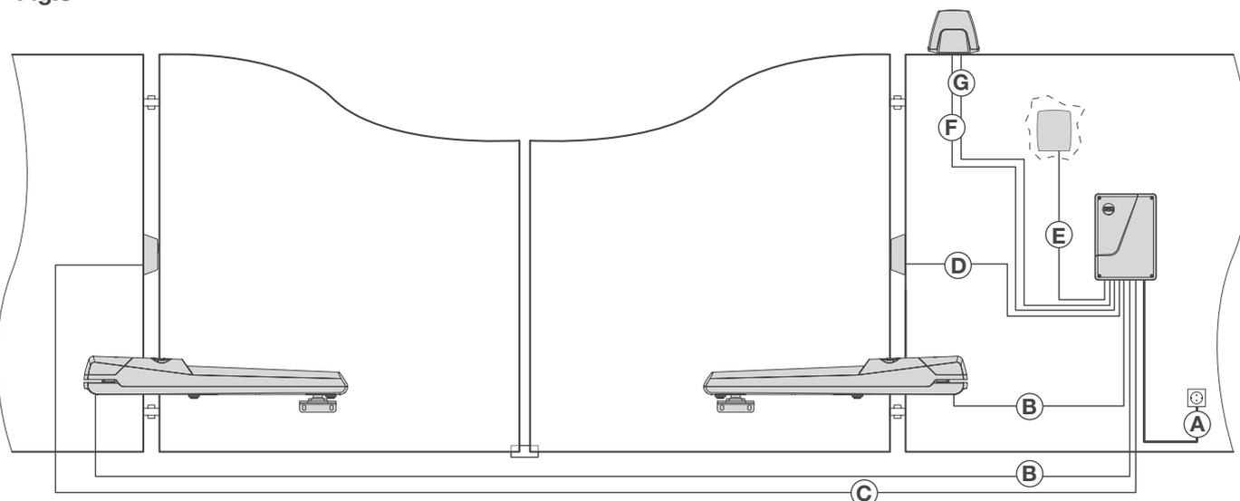
The cables necessary for the installation of BEAUTY can vary according to the accessories installed.
