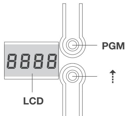
**i** With the display off, the "↑" button performs a Step-by-Step command. This function can be useful during the programming and inspection phases.
