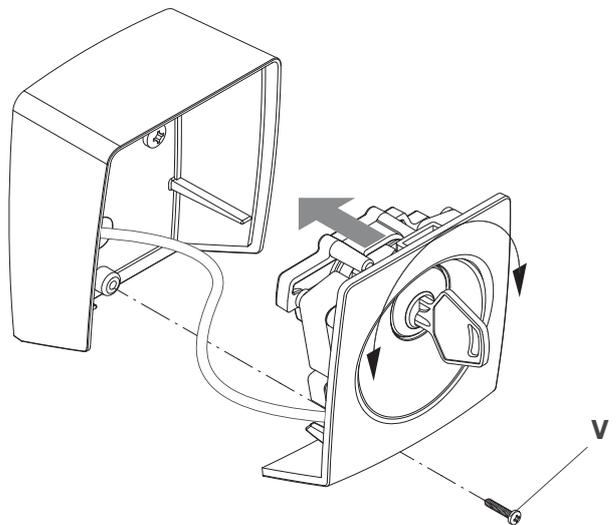
To close the selector, turn the key and hold it in this position, insert the selector into the base fixed to the wall. Release the key and fix the screw V.
