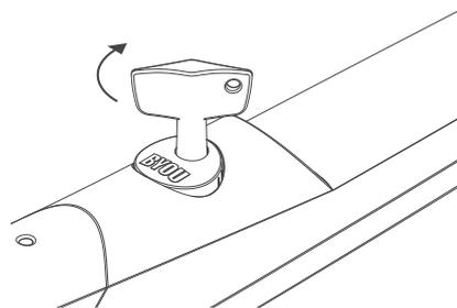
To go back to automatic functioning mode, put the release key back in the initial position, remove it and put the circular cover back in its initial position.
