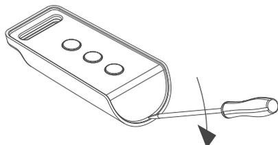
Use a small screwdriver as a lever in the zone indicated, in a way to open the transmitter.
