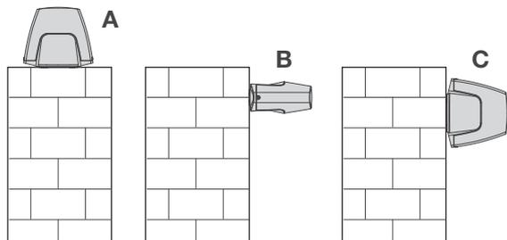
The flashing light can be fixed onto a horizontal or vertical surface. In the case of vertical installation the protection rating is reduced to X4.
