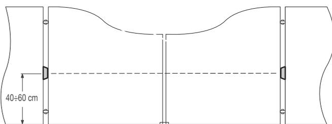
Trace the drilling holes using the photocell base as a reference.
