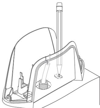
Trace the drilling points using the base as a reference. The central hole must correspond to the passage of the cables.
