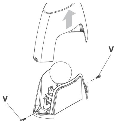
Loosen the two screws V and then remove the transparent cover.
