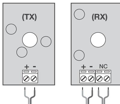
Make the connections and re-position the covers checking that the cover with the lens (RX - 4 clamps) is applied to the receiver. The lens can be recognised by the concentric circles that are visible in transparency.
