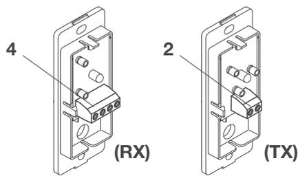
The two photocells must be fixed on the outside and as near as possible to the gate:
