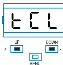
After accessing the BASIC MENU, press the + and – keys to scroll through the functions.
