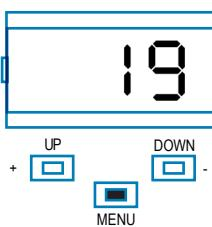
Press the MENU key for 1 second to display the parameter in order to save the modified value, or MENU quickly to quit the function without saving.
