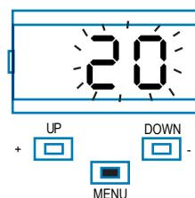
To access the value modification function, press the MENU key for 1 second, until the value starts to flash quickly.
