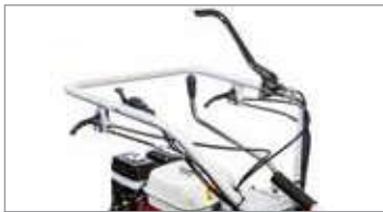
Steering with independently controlled releases and brakes.
