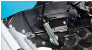
Direct gear selection lever located on the side of the steering column, for safe gear changes.
