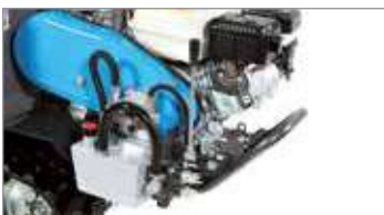
Lever-operated hydraulic tipping control valve.
