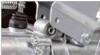
Handlebar mounted on vibration dampers.
