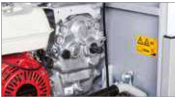
Independent PTO at 2100 rpm.
