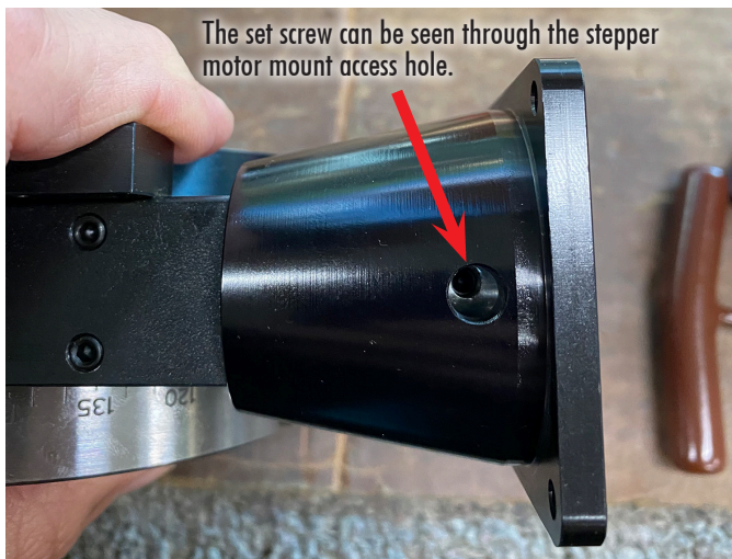
FIGURE 1—The set screw is aligned with the access hole.
