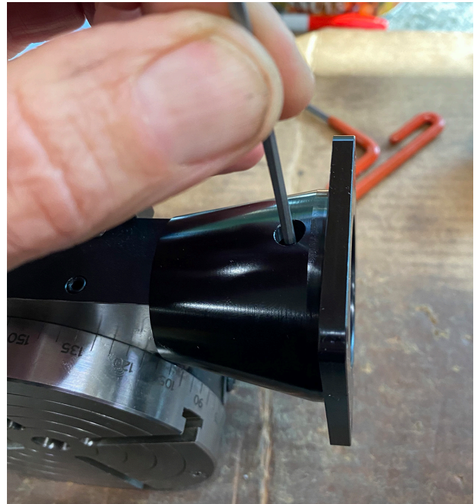
FIGURE 2—Shows the 3/32" Allen wrench inserted through the motor mount access hole.
