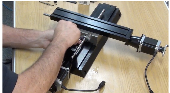
FIGURE 3—We highly recommend using a ball end Allen wrench to be able to get into the tight spaces.
