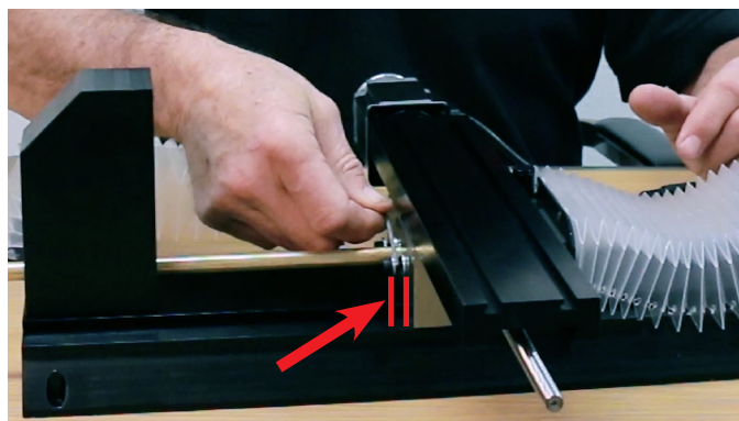
FIGURE 14—You can use your Allen wrench to create a gap between the washers that allows space for the front rear saddle mounting plate. The two red lines indicate the gap between the two washers on each 10-32 screw.
