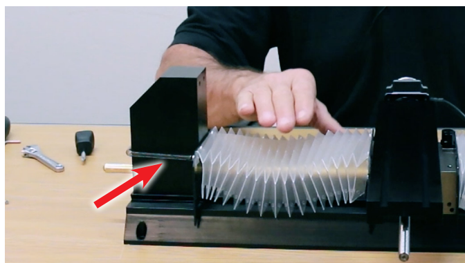
FIGURE 16—The red arrow is pointing to the spring that secures the back mounting plate to the mill column base.
