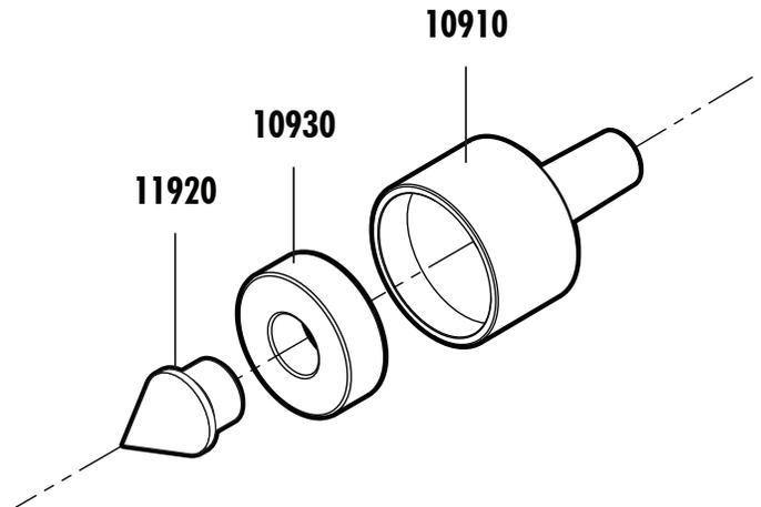
*Note: The bearing and nose piece are pressed in at the factory. Once assembled, the 1191 Live Center is not considered user-serviceable. Parts are shown for reference only.*
