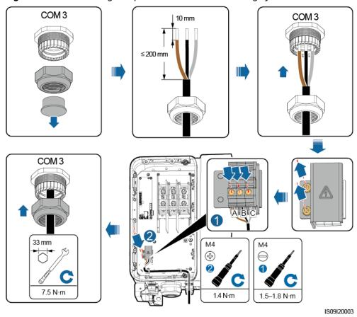
Figure 5-16 Connecting the power cable of the tracking system
