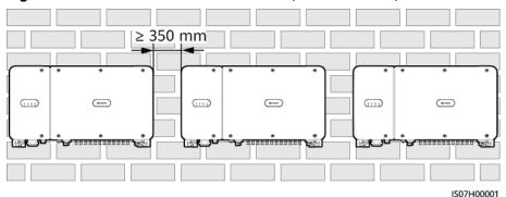
Figure 4-4 Horizontal installation mode (recommended)
