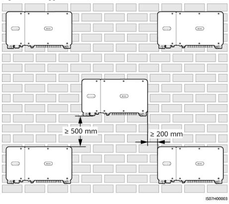
Figure 4-5 Staggered installation mode (recommended)
