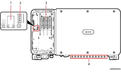
Figure 2-13 Wiring ports (SUN2000-100KTL-H0 and SUN2000-100KTL-H2)
