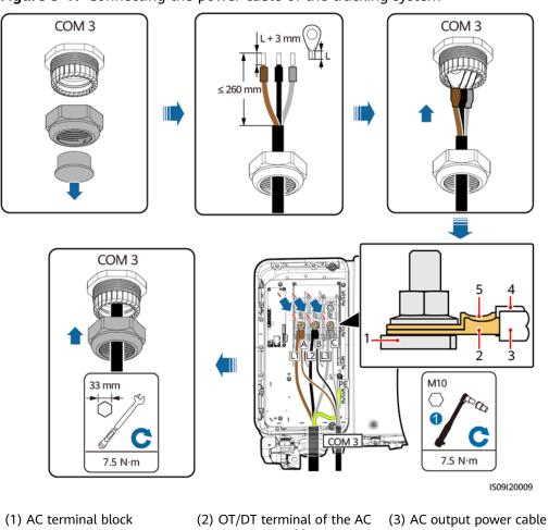
Figure 5-17 Connecting the power cable of the tracking system
