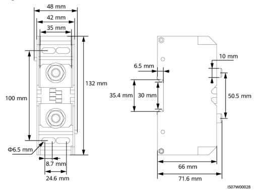
Figure 5-9 AC terminal block dimensions
