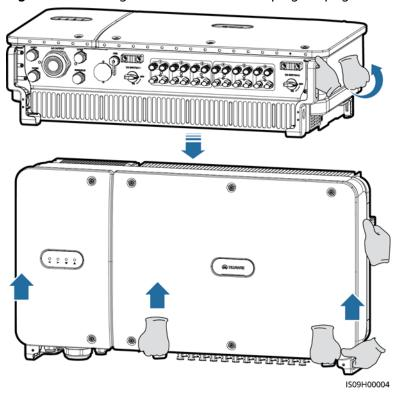
Figure 4-13 Lifting the SUN2000 and keeping it upright
