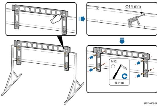
Figure 4-9 Installing the mounting bracket
