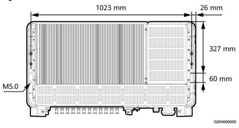
Figure 2-11 Dimensions of reserved holes on the rear
