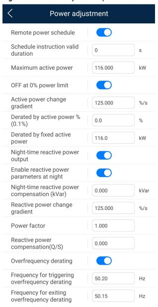
Figure 7-13 Power adjustment parameters
